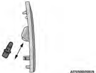
Front Side Marker Lamp Bulb Removal
