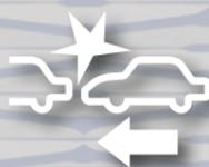
The **Pedestrian Emergency Braking (PEB) system** is a subsystem of FCW that provides audible and visual warnings, and may apply automatic braking when it detects a potential frontal collision with a pedestrian. You can turn the PEB system on or off through your radio.
