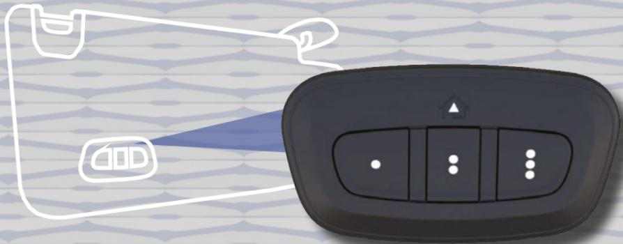
**1** While the car is ON, hold the handheld garage door transmitter 1-3 inches from the HomeLink® button you want to program in the vehicle.
